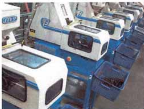
Micro-molding machines acquired with Matchless Molding range from 9 to 25 tons.
